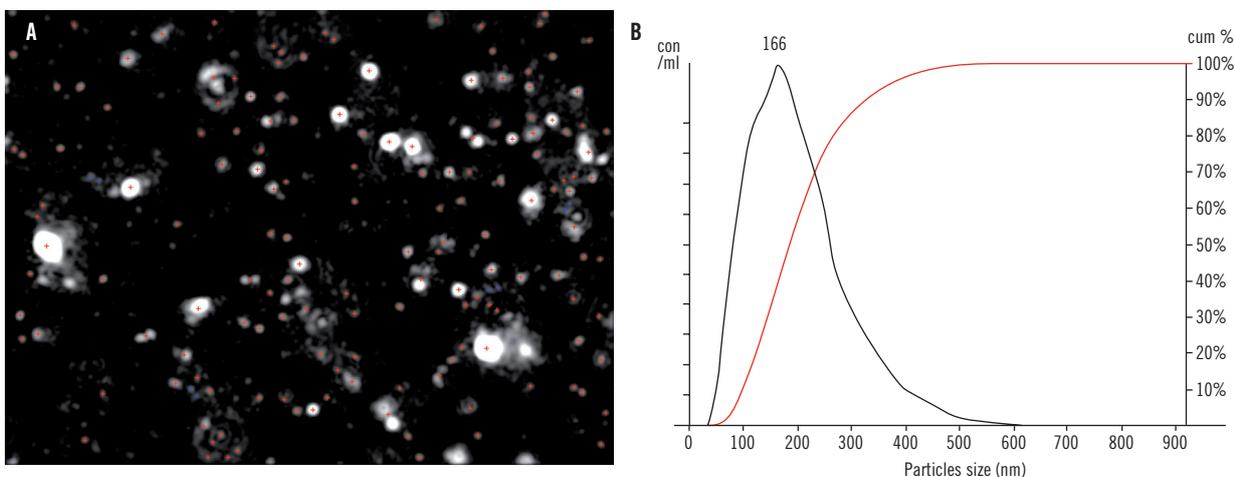
**Fig. 1** Exosome nanoparticle tracking (NTA). NTA is a light-scattering technique for rapid sizing and evaluation of extracellular vesicle concentrations, eg, of exosomes, which are visualized in **Panel A**. Distribution of the calculated vesicle size is shown in **Panel B**. Image and graph courtesy of Christian Harz, NanoSight Ltd.
